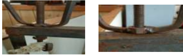
Fig.9. Clamp &amp; Screw arrangement
